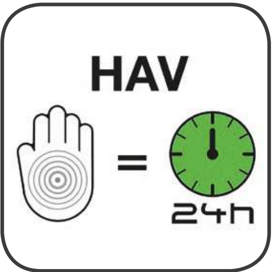
Low hand-arm vibration (HAV) values (< 5 m/s²) for working comfort even during prolonged application of the WP1550.
