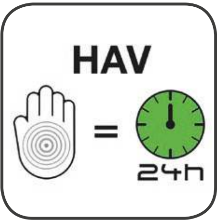
The hand-arm vibrations (HAV) are below 2.5 m/s² thanks to the vibration-reduced center pole, as a result the need for documentation lapses.
