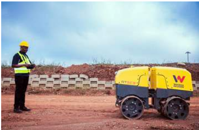
User safety: a proximity sensor between the operator and the machine automatically deactivates the machine within a range of 2 meters.
