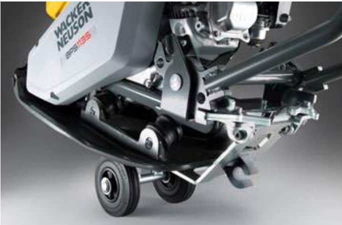
The wheel set (accessories) can be mounted easily. When folded down, the guide handle is automatically locked, and when folded up, released again.
