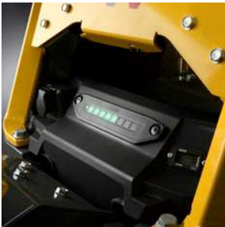
The compaction control Compatec supports daily work. With the optional Compamatic, compaction progress can be documented from a desk both comprehensively and fully.
