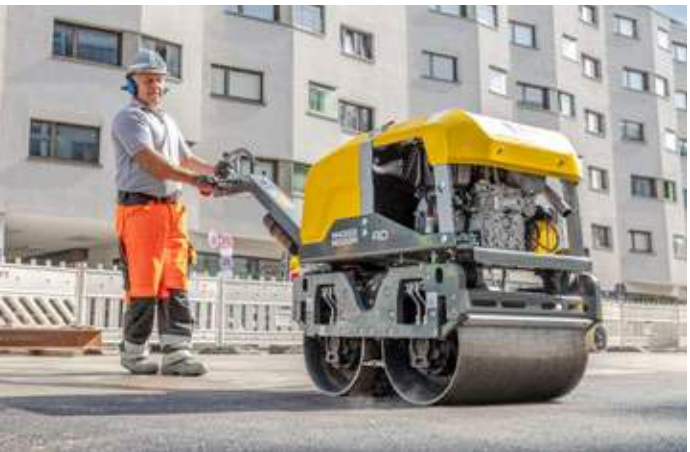
Long center pole facilitates steering and turning, especially in small areas.
