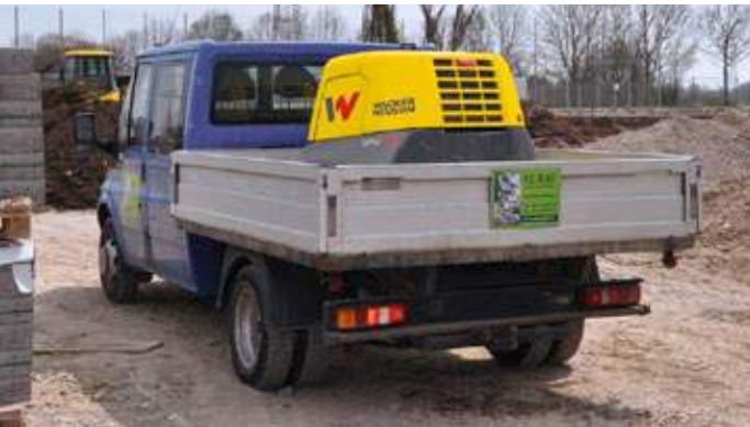
A low loader is not necessary: the DPU130r only weighs 1,200 kg and can be transported on a truck bed.
