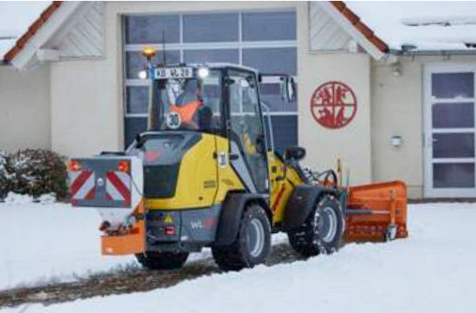
Winter road maintenance made easy with the snowplow and spreader.
